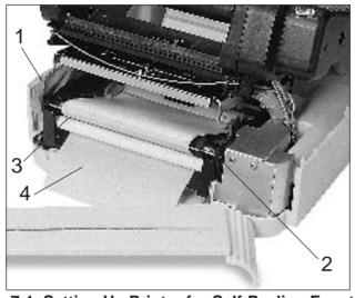
Fig. 7-1 Setting Up Printer for Self-Peeling Function
